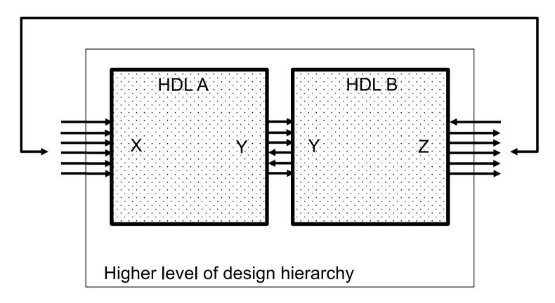
When verifying lower levels of hierarchy such as individual blocks of HDL, the verification engineer derives checkers from an understanding of the function, properties, and context of the larger design, e.g. from how the blocks will be used in the context of the design.
