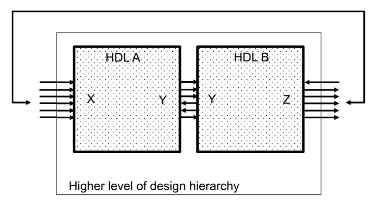
When verifying lower levels of hierarchy such as individual blocks of HDL, the verification engineer derives checkers from an understanding of the function, properties, and context of the larger design, e.g. from how the blocks with be used in the context of the design.
